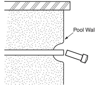
2. Use Inside Pipe Cutter (part #5-17-4) to cut pipe back 5/8" behind shell surface.
