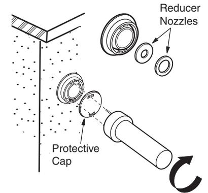
5. At startup, select and insert the applicable restrictor nozzle if required for the installation.
