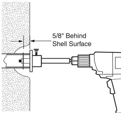
3. Prime pipe and fitting. With protective cap attached, glue fitting into pipe, positioning for thickness of finish material.
